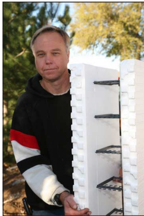
Marc Robinson , president of MDR Construction, Inc., holds an ICF, an Insulated Concrete Form, which is an expanded polystyrene material that is stacked up and becomes the wall in a concrete house after concrete is poured down the interior of the form. This makes a wall that is almost eleven inches thick.
