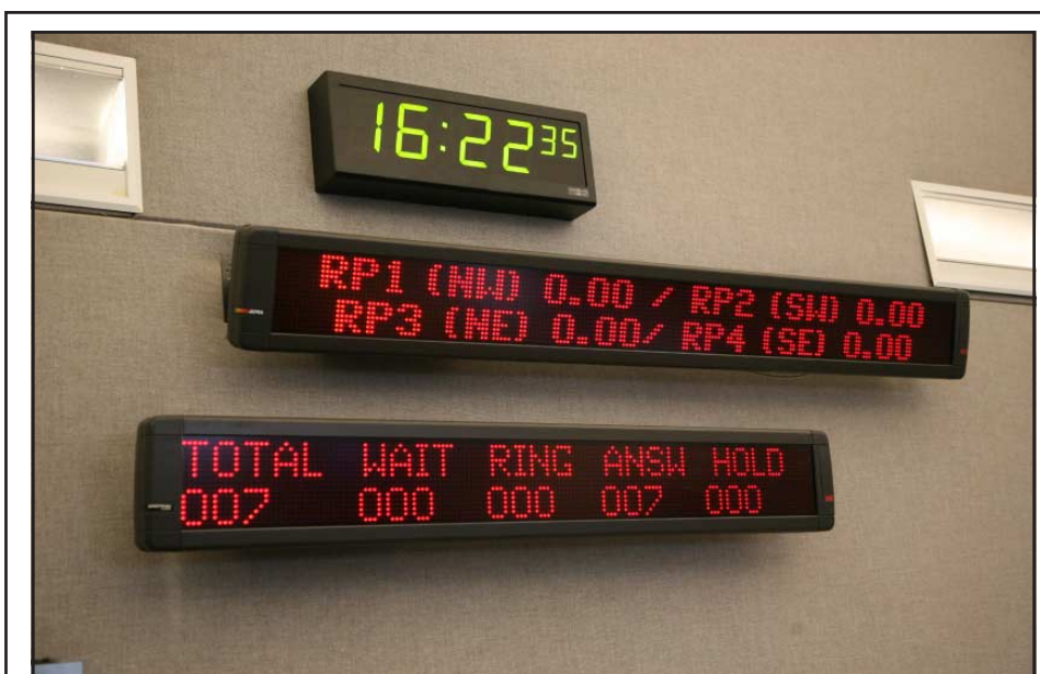
The message board gives a quick overview of the level of activity going on in the message center. The top area deals with police response time and bottom area deals with the status of incoming calls and response, all these functions are controlled and tallied via computers. Chris Martin said, "Operators are frequently rotated for cross-training purposes." The telecommunicators stay in their area but rotate break schedules and stations. There are four telecommunicator pods with a total of 15 stations.
